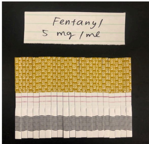
Figure 7 Fentanyl. Negative results were observed in Cal 5 (5 mg/mL). The remaining tests were not performed.
